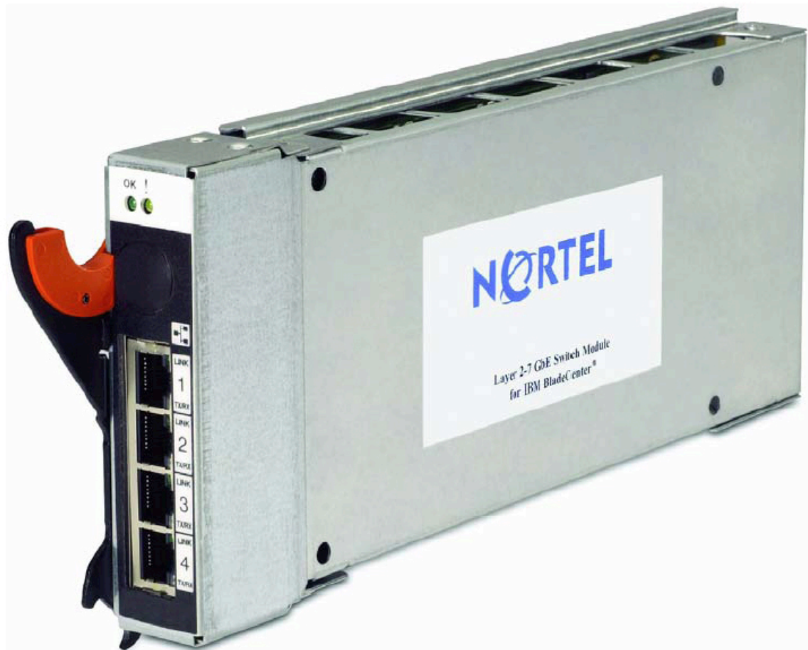
Figure5 – The Nortel Layer2-7 GbE Switch Module blade includes four external 1000BASE-T connectors for up to 4 gigabit/sec. Ethernet connections, 14 internal full-duplex gigabit ports, one for each blade server in a BladeCenter chassis, management support for Spanning Tree Protocol and SNMP protocols and serial port for software installation and configuring.
